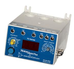
SymCom's Model 777-P2 is a fully programmable electronic overload relay. It is designed to monitor and protect any 3-phase, 200-480VAC motor drawing 2-800 full load amps (external CTs are required above 90 amps). It provides unsurpassed protection from faulty voltage, underload and overload conditions.
